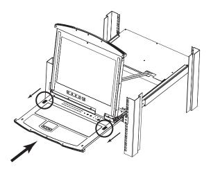
2. Let go of the catches. Using the front handle, push the keyboard module all the way in.
